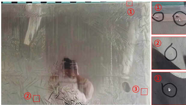
Figure 5. Photography of panel failure after LLO process.
